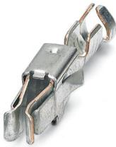
Module female contact, is inserted into the plug housing MSTBC after crimping the conductor, for conductors from 0.5 to 1.0 mm<sup>2</sup>
